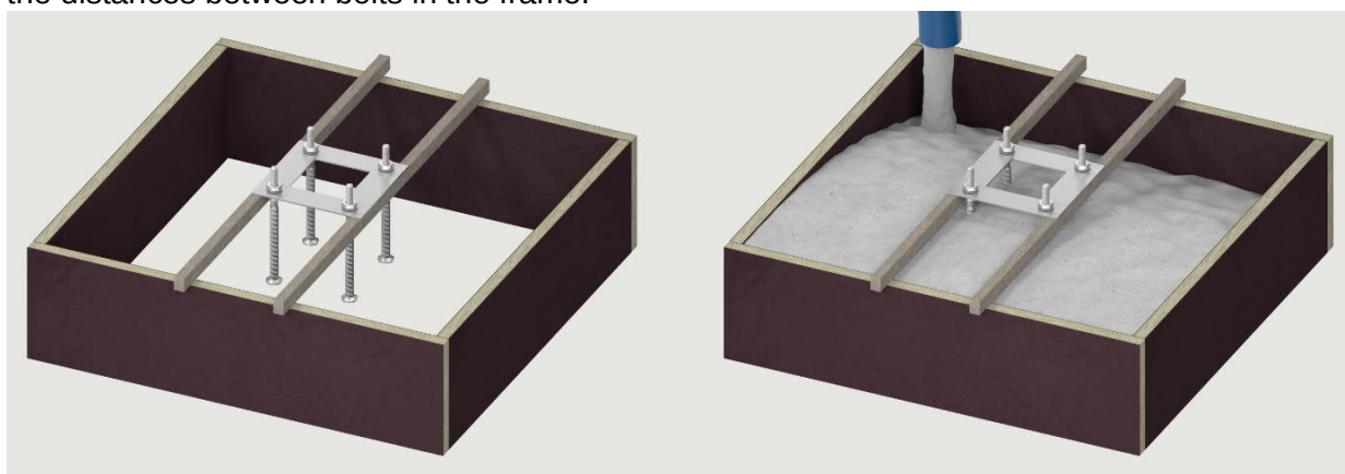
Figure 29. Installing the bolts using a frame and casting the foundations
